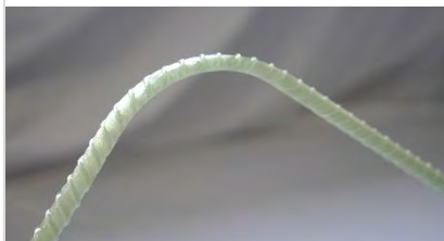
Formed reinforcing bars made from fiber-reinforced plastics (glass and carbon fiber)
