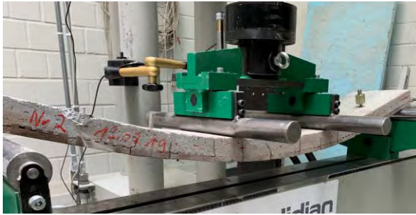
Figure 29: Two-point bending test on a slab strip with non-metallic reinforcement
