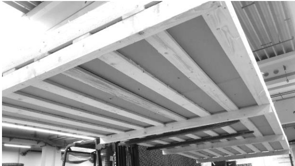
Figure 9: Pallet transport for flat reinforcement grids
